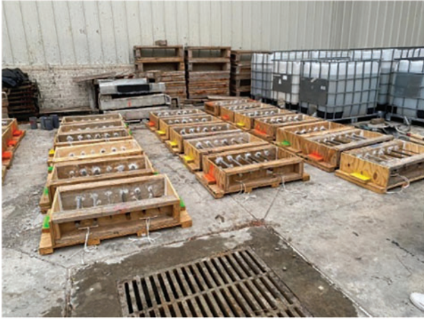
Figure 1. Sample preparation: formwork
