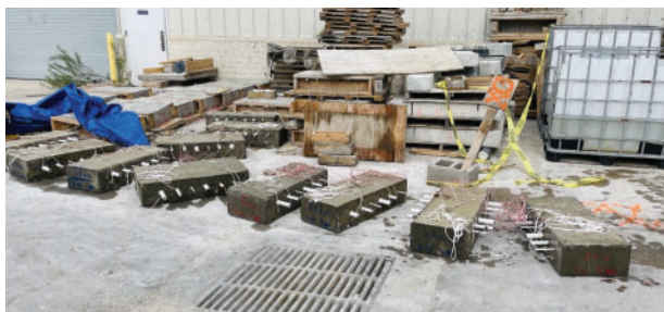
(a) Accelerated corrosion process
