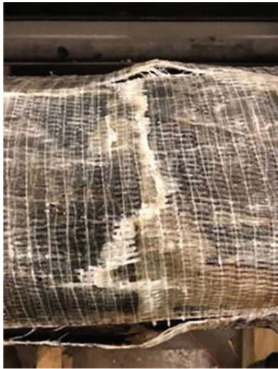
Figure 20. FRP splice cracking under applied load at top
