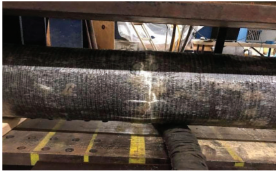
Figure 25. Bulging in FRP splice under compression. FRP, fiber-reinforced polymer
