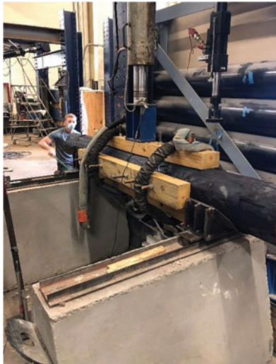
Figure 3. Shear test setup with wooden splice
