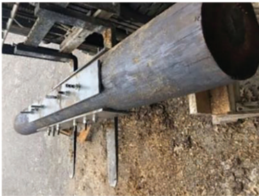
Figure 2. Steel plate splice specimen
