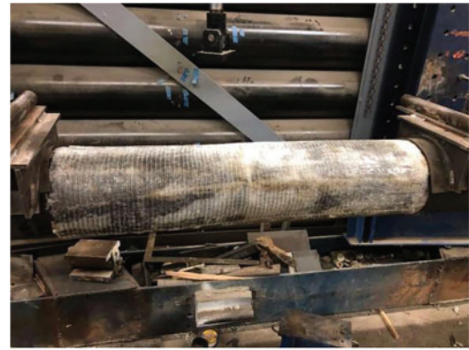
Figure 4. Finished pile with glass fiber-reinforced polymer composite splice
