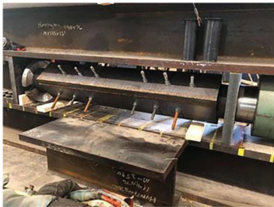
Figure 9. Axial test setup with C-channel splice
