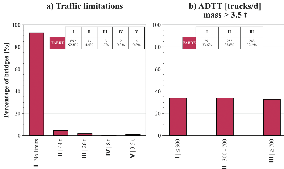
Figure 6. Frequency histograms of the parameters involved in Structural-foundational Hazard Class : (a) Traffic limitations and (b) Average Daily Truck Traffic (ADTT). The absence of traffic limitations would result in higher hazard classes, but, conversely, low ADTT values reduce the hazard classification. Overall, 93.2% of bridges are classified with a High or Medium-High hazard (Fig. 5). This increases the likelihood that the Structural-Foundational Warning Class , at the end of the calculation, will be High or Medium-High , which entails a significant number of accurate assessments and more frequent periodic inspections
