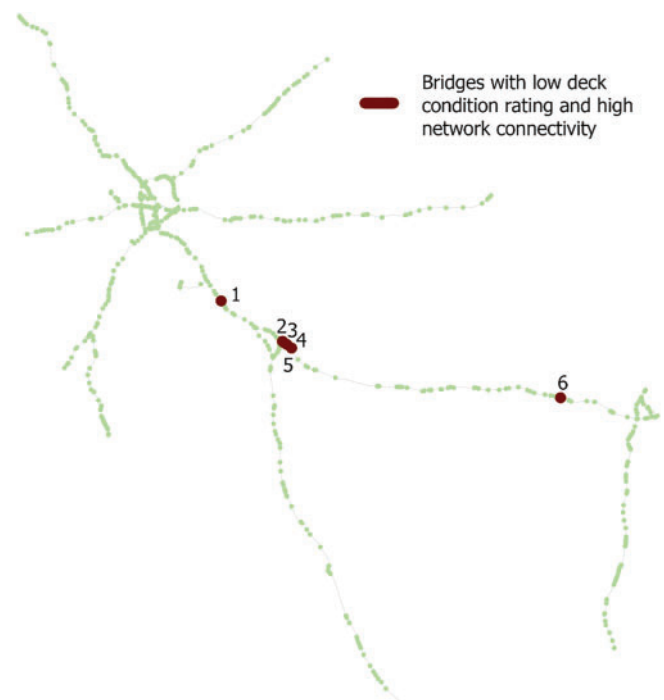
Figure 16. Bridges with low deck condition ratings that play a major role in network connectivity
