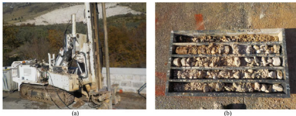
Figure 3. Example of vertical coring (Bridge on SP9 in Caserta Province): (a) coring machine and (b) extracted material
