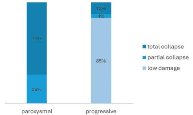
**Figure 15.** Probability of damage evolution in bridge–landslide interaction mechanisms: paroxysmal vs. progressive
