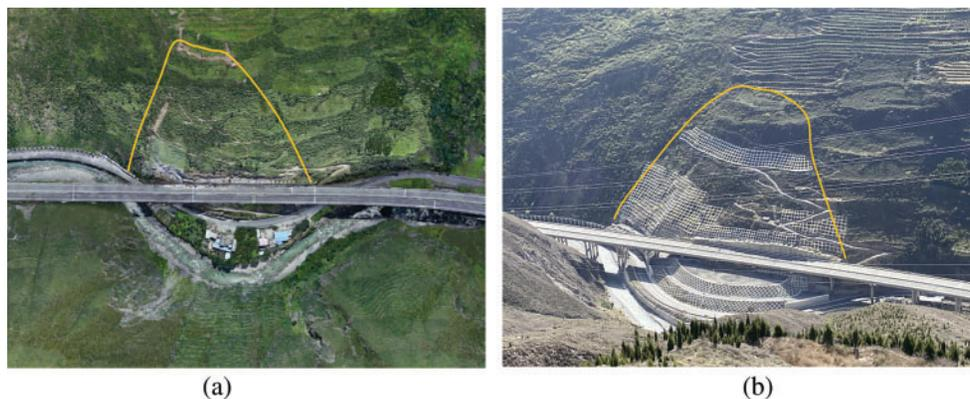
**Figure 8.** Landslide along the Wenchuan-Maerkang highway, Li County, China. (a) Aerial view of June 2020 and (b) April 2023 after reprofiling and stabilization works (courtesy of Kun He, adapted from Du et al.<sup>29</sup>)
