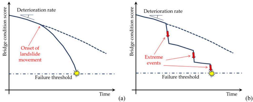
**Figure 14.** (a) “Progressive” and (b) “Paroxysmal” evolution of bridge degradation over time
