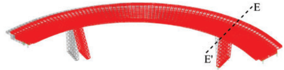
Figure 15. A deformed configuration of the numerical model of the case study bridge, obtained by simulating the evolution of the mountain landslide with the indicated section of the deck triggering the collapse condition
